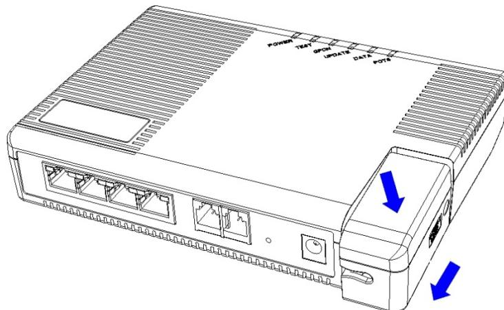
Figure 7: Remove the Laser Lock Door
