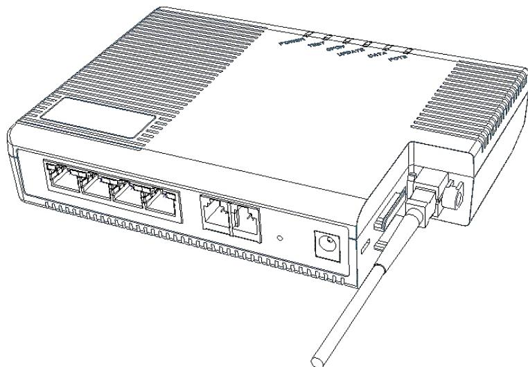
**Figure 8: Plug in the fiber connector**
