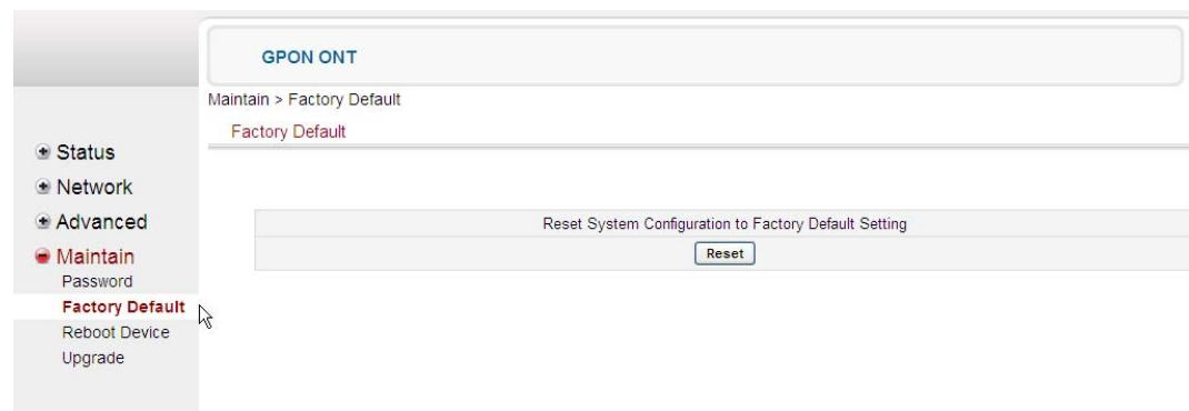
**Note:** In addition to using this screen, the system configuration can be reset to the factory default values by pressing the Reset button on the back of the B-FOCuS for more than 5 seconds.
