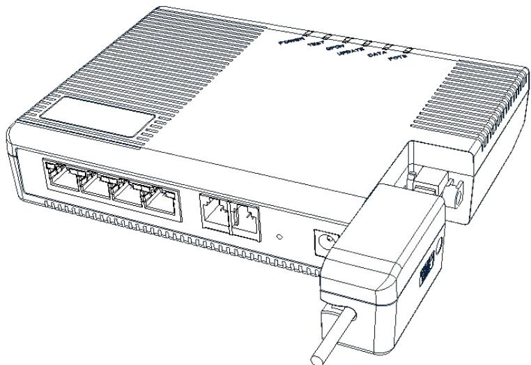
**Figure 9: Attach the Laser Lock Door**
