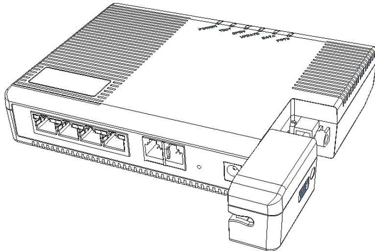
3. Remove the dust covers from the SC/APC optical connectors. Clean the connector if necessary.
