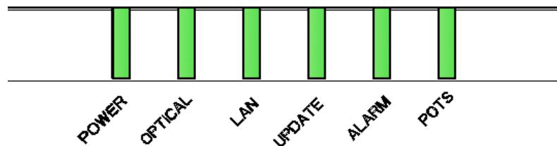
Figure 12: B-FOCuS O-4F2P Status LEDs location
