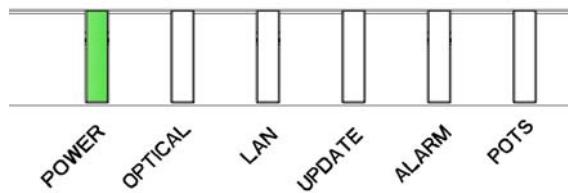
**Figure 10: B-FOCuS O-4F2P has not yet been provisioned**
